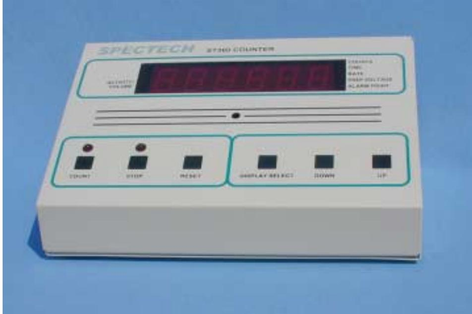
The ST360 Radiation Counter combines many features into a single inexpensive instrument. The classic nuclear scaler design has been expanded to include a preset time function, a digital rate-meter with alarm, a digitally controlled high voltage supply, and computer interfacing via RS232 serial or USB formats.
