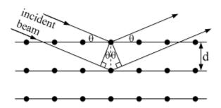
Figure 2. Electron Waves Reflected from Atomic Planes.
