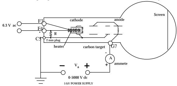
Figure 4. Electron Diffraction Experiment Diagram.
