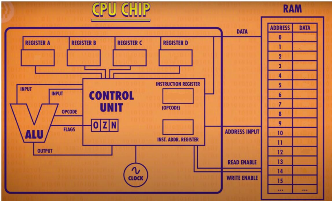
FIGURE 1. Layout for a theoretical 4-bit CPU.
