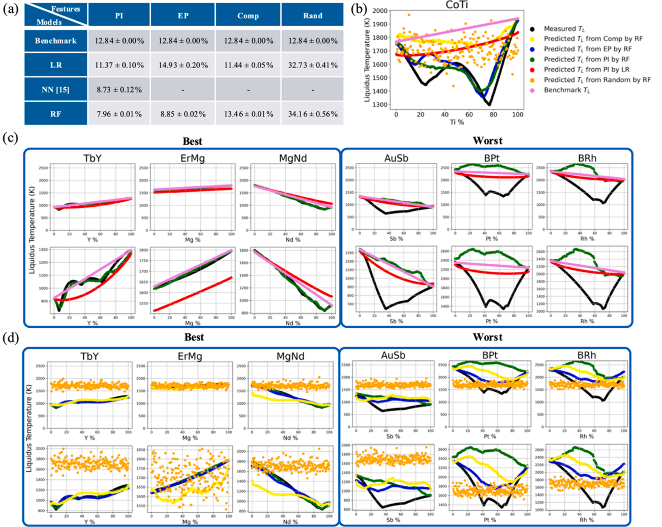
Fig. 3. Summary of the ML predictions of T_L for binary alloys: (a) Summary of average predictions from linear regression, neural network and random forest with 10-fold CV where training/testing data splitting is based on alloy systems. The benchmark model (linear interpolation), T_{avg} = p_A \cdot T_A + p_B \cdot T_B , is also shown. Standard deviations are given over five trials for all models. (b) Random forest predictions of T_L using four different features vectors (Comp, EP, PI, Random) for Co-Ti as an example binary alloy. These predictions are compared to T_L obtained from the linear regression and benchmark models. The best prediction, quantified by the lowest MAPE of \sim 4\% is obtained using the random forest model trained on PI features. EP features result in a MAPE of \sim 5\% . Composition features result in a MAPE of \sim 15\% and random features result in a MAPE of \sim 12\% . (c) Three examples are shown of the most accurate and least accurate predictions for an alloy system (top images are all at same temperature scale, bottom images are zoomed in at different scales) with Physically Informed features, the leave-one-system-out validation method and different models. The best three alloy systems prediction are for TbY (MAPE = 0.41%) and ErMg (MAPE = 1.37%) and MgNd (MAPE = 2.25%). The three worst predictions for alloy systems are for BRh (MAPE = 44.61%), BPt (MAPE = 44.27%) and AuSb (MAPE = 38.00%). These worst predictions are even worse than the predictions using the benchmark model. (d) Three examples of the most accurate and least accurate Random Forest predictions for an alloy system (top images are all at same temperature scale, bottom images are zoomed in at different scales) with different features and the leave-one-system-out validation method. The PI features give the best predictions.
